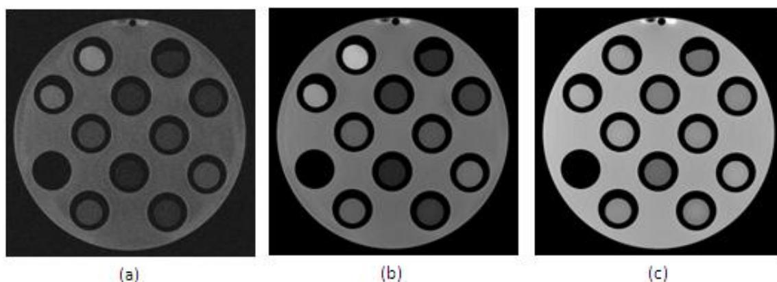
Figure 5: Spin-Echo DICOM series with repetition times of 200 ms (a), 400 ms (b), 2 s (c).
