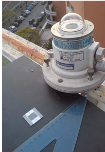
Figure 4: A polysulphone dosimeter on the left side, a broad band radiometer on the right side (Solar Radiometry Observatory, “Sapienza” Università di Roma)
