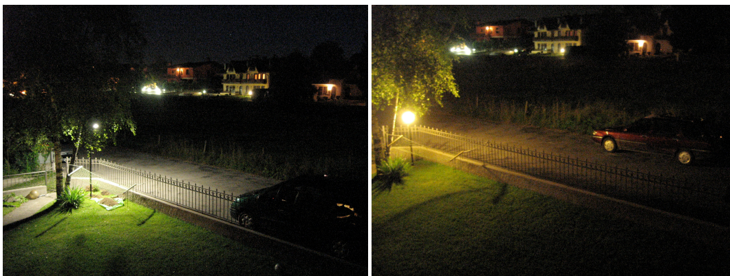
Figure 1: Left: Night illumination of a garden with a semi-cutoff fixture; the eye is not dazzled by the lamp. Right: the same garden with a simple ball fixture; the eye is strongly dazzled by the lamp.
