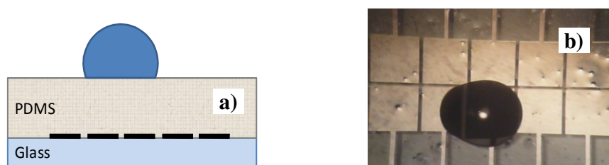
Figure 3. a) Cross section of the EWOD device. b) Frame showing the deformation of the droplet during the movement.
