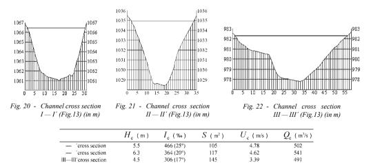
Tab. 2 - Shape parameters of cross section and estimated velocities and peak discharges of debris flows in Mozi gully
