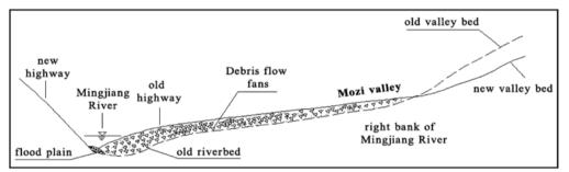
Fig. 15 - Comparison of landform change before and after debris flow events in Mozi gully
