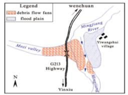
Fig. 17 - Sketch map of Mingjiang River blocked by debris flow from Mozi gully in December, 2008
