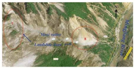
Fig. 8 - Aerial image Showing two of the eight landslide dams in Mozi gully after the earthquake (Scale:5000) (2008.6, National Geomatics Center of China)
