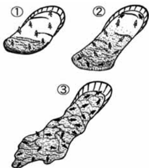
Fig. 5 - Classification of landslide masses by movement mode
