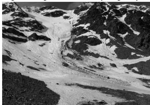
Fig. 4 - 15 July 2008. The Western Korgashinlitau glacier. The source of the Rakyt-1 river: 1 – the area of origination of the 2 August 2007 debris flow and the path of movement of outburst water masses from an intraglacial hollow; 2 – the outflow grotto, formed in 2008
