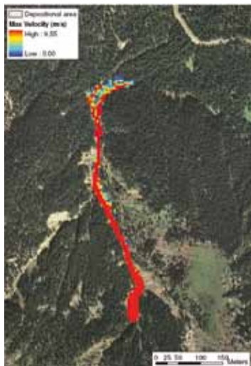
Fig. 8 - FLATModel simulation result in the Ensija's Catchment. Maximum velocity recorded during the simulation
