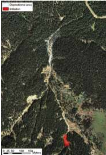
Fig. 7 - Initiation and depositional areas of debris flow for the event of 2006 in the Ensija's Catchment
