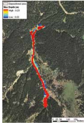
Fig. 9 - FLATModel simulation result in the Ensija's Catchment. Maximum depth recorded during the simulation
