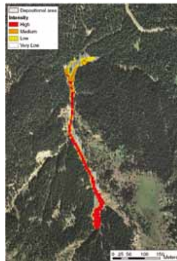
Fig. 10 - Result of the intensity analysis using the output of FLATModel
