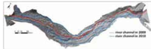
Fig. 10 - The evolution of gully channel configuration caused by debris flows in 2009 and 2010
