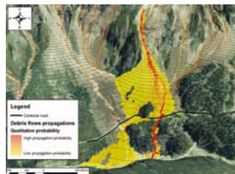
Fig. 9 - Example of spreading assessment in the Mauvoisin region. A documented spreading zone is highlighted, but the model identified a source area and their respective propagation for every torrent (modified after JABOYEDOFF et alii, in review)
