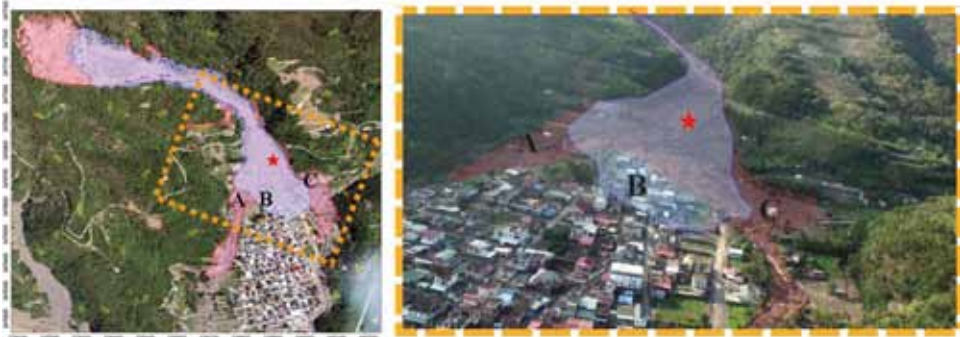
Fig. 13 - Region in red is area affected by Typhoon Morakot, and the blue region is the simulation result. The red star indicates where field depth estimation is available. The depth estimated by rescuer is between 12 m and 13 m. The simulated result for 50,000 m 3 is 13 m
