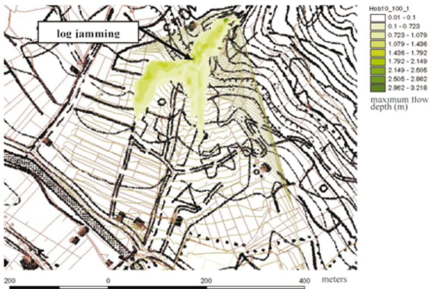
Fig. 7 - Maximum simulated flow depth for a debris-flow volume of 10 000 m 3 , a peak discharge of 100 m 3 /s and a \tau_c/\rho = 1.0 \text{ m}^2/\text{s}^2 ratio assuming log jamming of the stream at the apex of the alluvial fan
