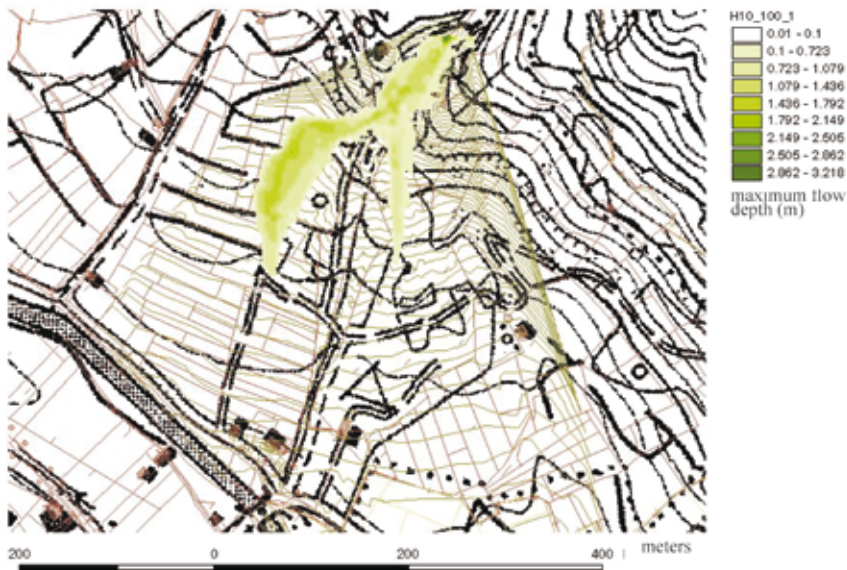
Fig. 4 - Maximum simulated flow depth for a debris-flow volume of 10 000 m 3 , a peak discharge of 100 m 3 /s and a \tau_c/\rho = 1.0 \text{ m}^2/\text{s}^2 ratio
