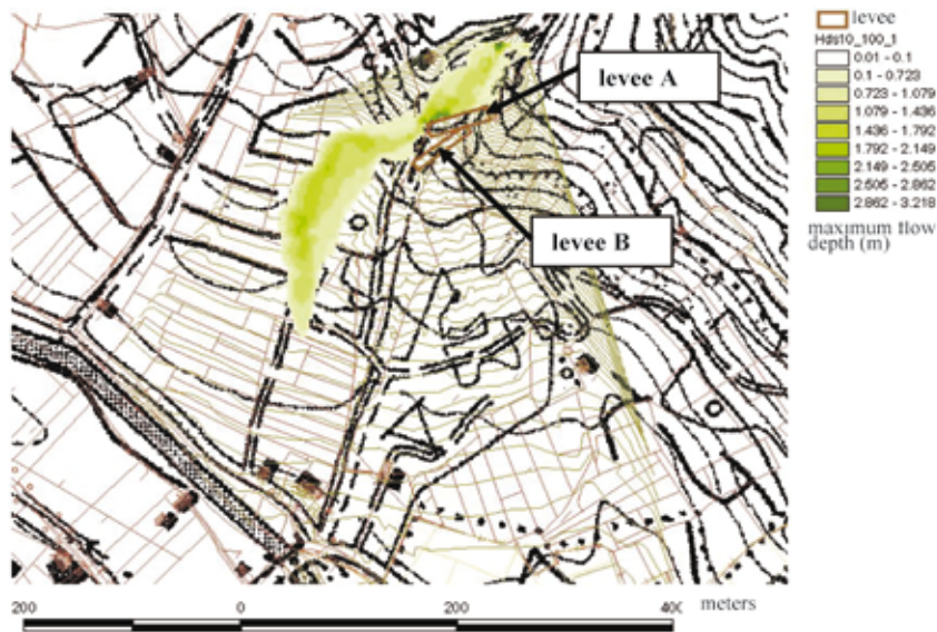
Fig. 8 - Maximum simulated flow depth for a debris-flow volume of 10 000 m 3 , a peak discharge of 100 m 3 /s and a \tau_c/\rho = 1.0 m 3 /s 2 ratio assuming the presence of a protection levee showing a 45° angle with the channel axis
