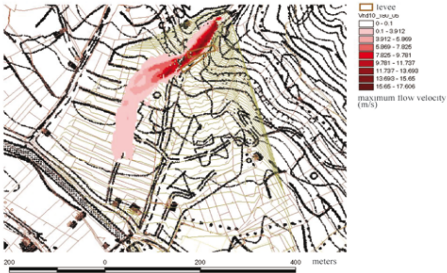
Fig. 9 - Maximum simulated flow velocity for a debris-flow volume of 10 000 m 3 , a peak discharge of 180 m 3 /s and a \tau/\rho = 0.5 m 2 /s 2 ratio assuming the presence of a protection levee showing a 15° angle with the channel axis
