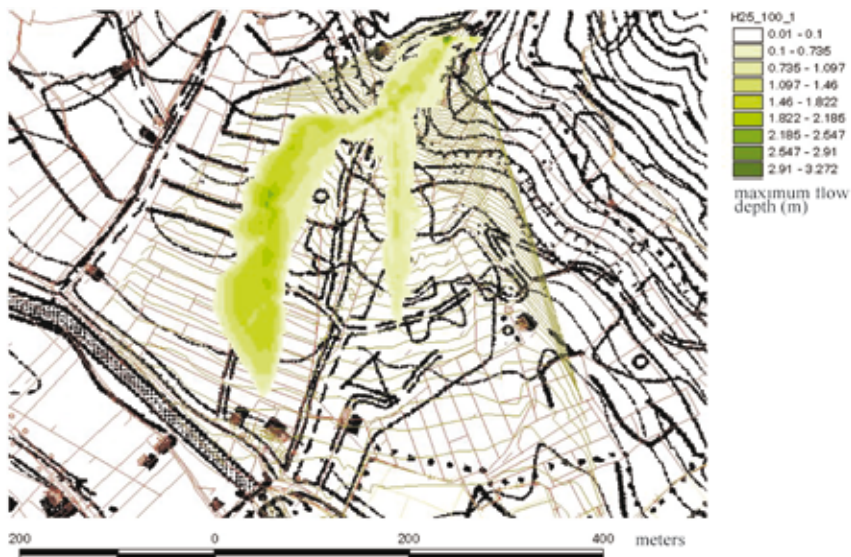
Fig. 5 - Maximum simulated flow depth for a debris-flow volume of 25 000 m 3 , a peak discharge of 100 m 3 /s and a \tau/\rho = 1.0 m 2 /s 2 ratio
