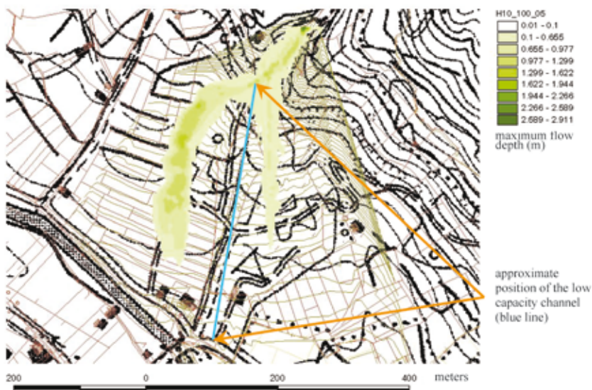
Fig. 3 - Maximum simulated flow depth for a debris-flow volume of 10 000 m 3 , a peak discharge of 100 m 3 /s and a \tau_0/\rho = 0.5 m 2 /s 2 ratio
