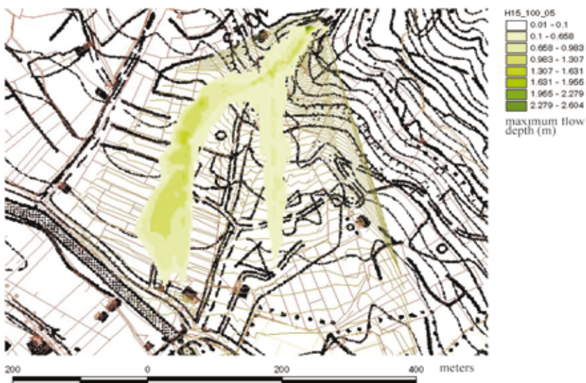
Fig. 6 - Maximum simulated flow depth for a debris-flow volume of 15 000 m 3 , a peak discharge of 100 m 3 /s and a \tau/\rho = 0.5 m 2 /s 2 ratio
