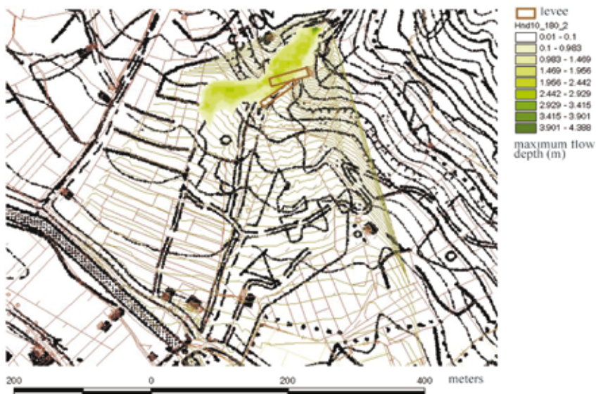
Fig. 10 - Maximum simulated flow depth for a debris-flow volume of 10 000 m 3 , a peak discharge of 180 m 3 /s and a \tau/\rho = 2.0 m 2 /s 2 ratio assuming the presence of a protection levee showing a 15° angle with the channel axis
