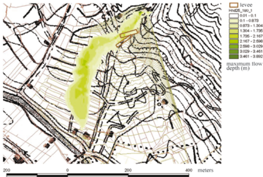
Fig. 11 - Maximum simulated flow depth for a debris-flow volume of 25 000 m 3 , a peak discharge of 180 m 3 /s and a \tau_c/\rho = 1.0 m 2 /s 2 ratio assuming the presence of a protection levee showing a 15° angle with the channel axis
