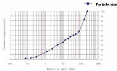
Fig. 12 - Curve of particle size distribution for sieve analysis of the field sample
