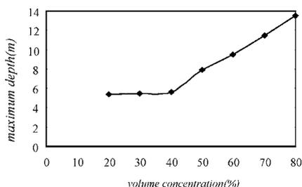
Fig. 14 - The relationship of volume concentration and maximum depth with the debris flow
