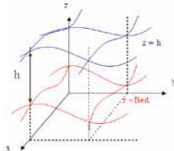
Fig. 1 - Definition of coordinate system for two-dimensional governing equations
