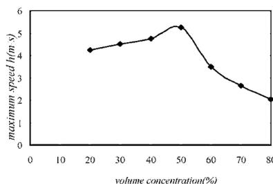
Fig. 15 - The relationship of volume concentration and maximum speed with the debris flow
