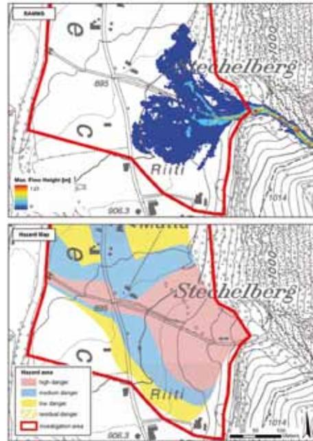
Fig. 2 - Debris flow modelling with RAMMS and hazard map, 300-years scenario (Map UP5<sup>®</sup> Office for Geographical Information Canton Bern)
