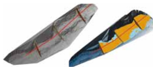
Fig. 7 - 3-D Model of the Merdenson torrent with empty barriers (left) and filled barriers (right)
