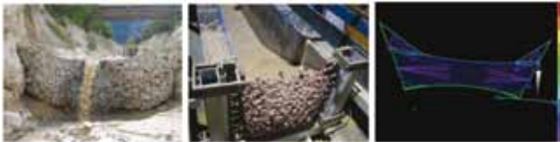
Fig. 2 - Development of a load model for flexible debris flow barriers: Field tests in the Illgraben (left), physical modelling with small scaled tests in the laboratory (centre) and numerical modelling with the finite element software (right) (WENDELER, 2008; VOLKWEIN, 2004)
