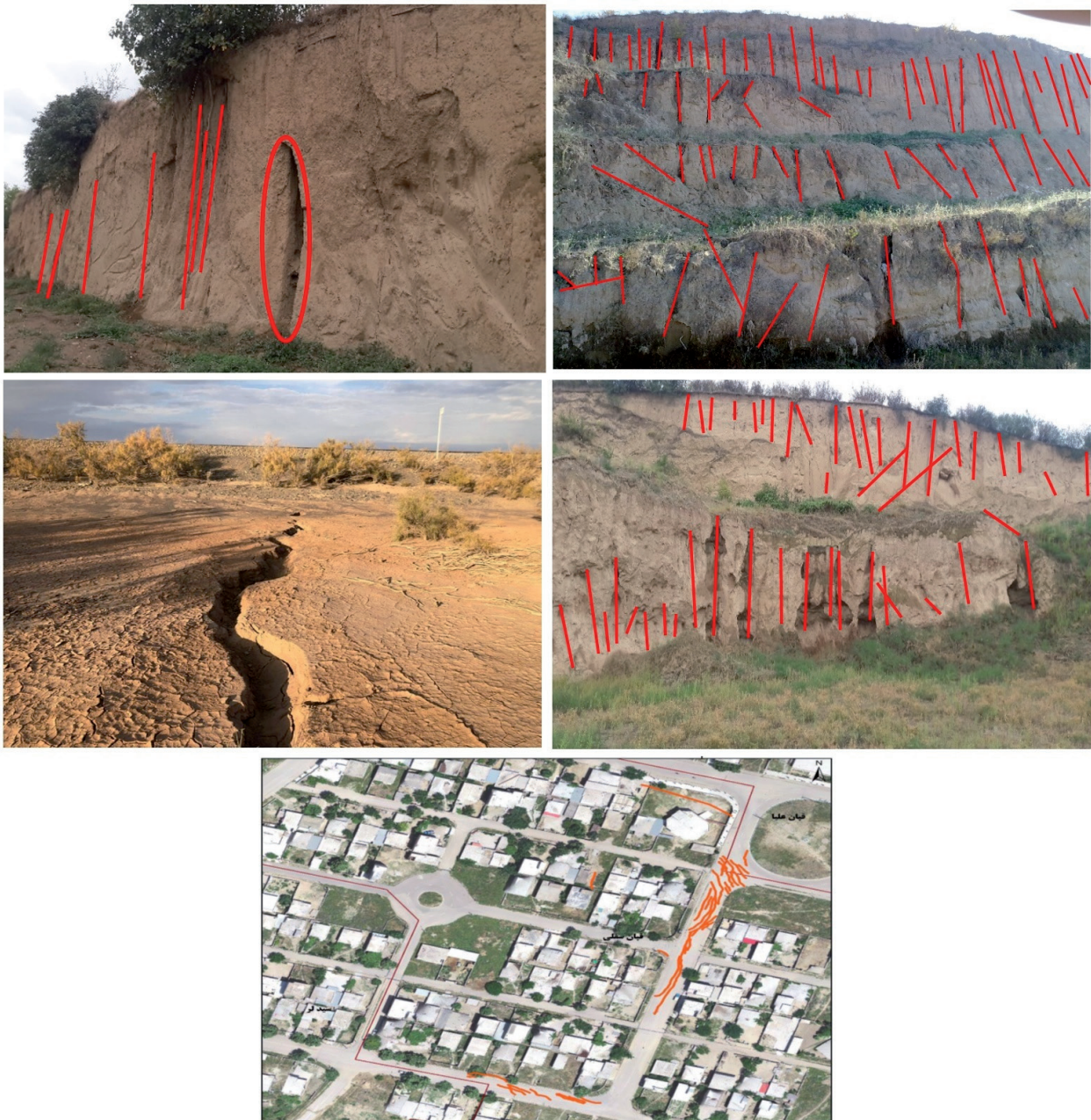
Fig. 4 - Joints in loess plateau: a) The effect of tree roots on crack propagation (Sad Abad) b) Nearly parallel and equally spacing joint development (Seyyed Miran) c) Surface water accumulation and formation of mud cracks and joints (Alagol) d) Washing holes developed along the vertical joints, and vertical joints developed on the back scarp of the loess caves e) Ground cracking due to soil collapse (Ferraghi city).
