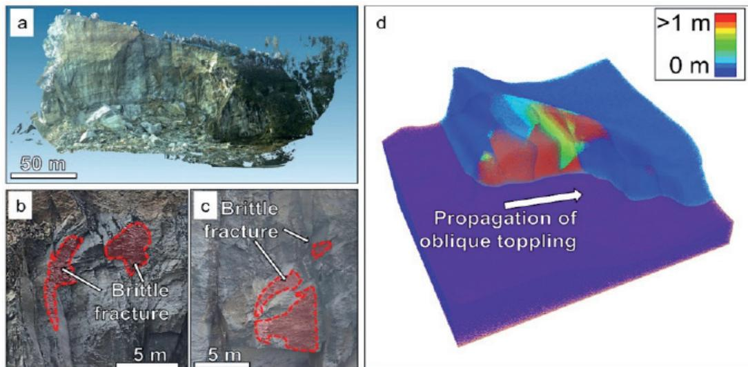
Fig. 3 - Overview of the Slope damage analysis at the San Leo landslide site. a: 3D model of the landslide scar from Structure-from-Motion. b,c: examples of brittle damage features observed across the scar, characterized by rough surfaces connecting structural discontinuities. d: Numerical modelling of the San Leo landslide. The progressive, brittle propagation of discontinuities caused the initiation of an oblique toppling failure that progressed from East to West (view of the model from North)
