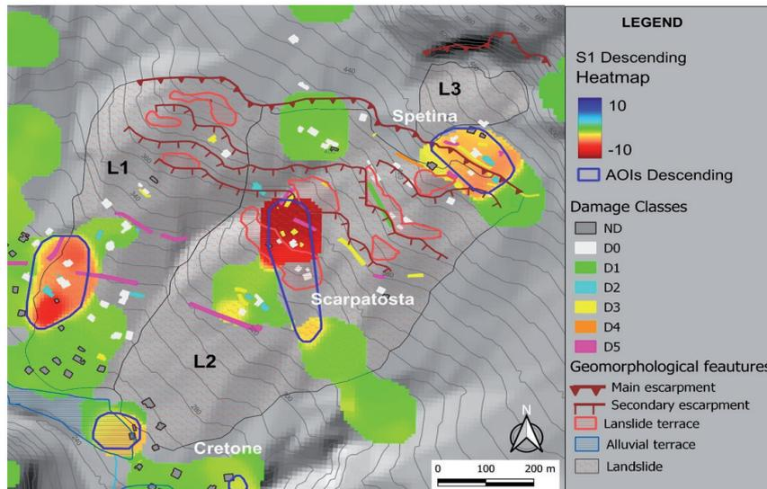
Fig. 5 - Sentinel-1 heatmap (descending) and AOIs in the Belmonte Castello area. The landslide perimeters L1, L2, and L3 defined by this work have been represented in grey; damage classes of the surveyed buildings and walls are ND= not defined; D0= negligible, D1= very slight, D2= slight, D3= moderate, D4= severe, and D5= very severe
