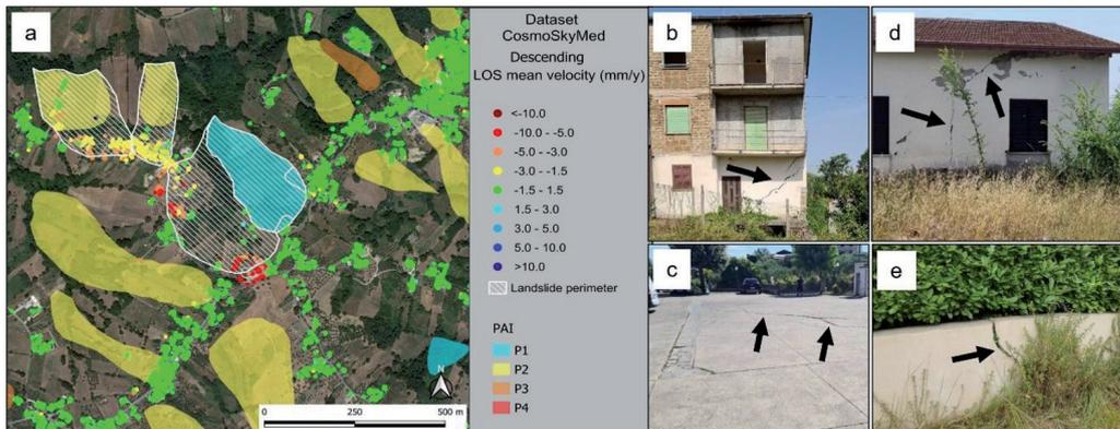
Fig. 7 - a) COSMO-SkyMed LOS velocity map (descending), with inventoried landslides from the PAI catalog, in the Strangolagalli municipality (Central Italy). The landslide perimeter defined by this work has been represented in white; b, c, d, e) photographs of the cracks on the most damaged buildings, roads, and walls
