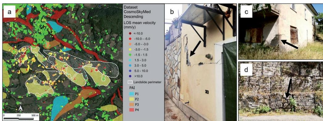
Fig. 9 - a) COSMO-SkyMed LOS velocity map (descending), with inventoried landslides from the PAI catalog, in the Arpino municipality. The landslide perimeters defined by this work have been represented in white; b, c, d
