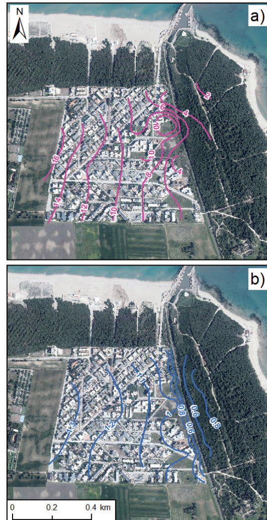
Fig. 2 - a) Thickness (in m) of the sandy soils covering the Lesina Marina chalky deposits (modified from FIDELIBUS et alii , 2011); b) groundwater level in m a.s.l. (modified from CAPORALE et alii , 2013). Basemap: 2019 aerial photo from https://www.sit.puglia.it/portal/portale_cartografie_tecniche_tematiche/WMS
