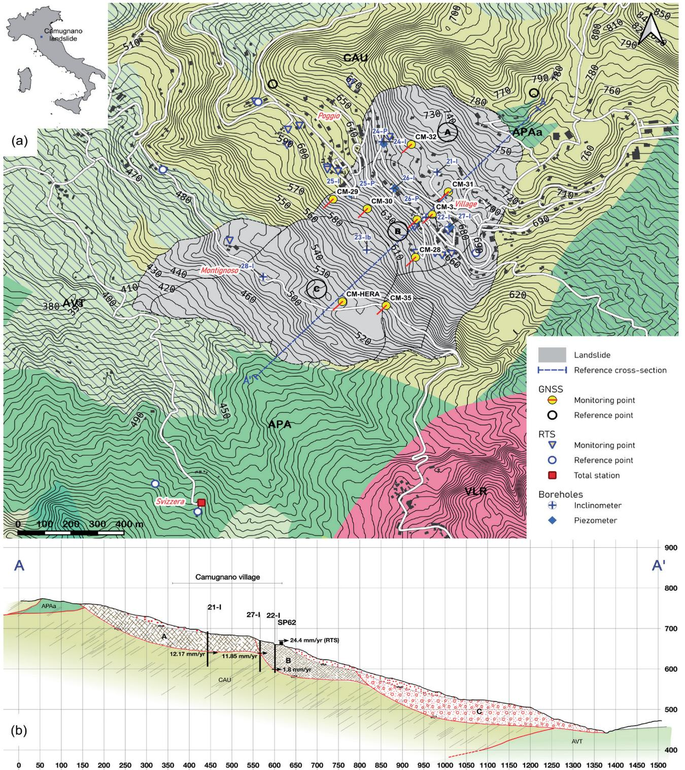
Fig. 1 - - Camugnano landslide. (a) reference map; (b) cross section. Letters A, B and C refer to landslide units mentioned in the text. Bedrock geology: Camugnano Formation (CAU), Argille variegate di Grizzana Morandi (AVT), Argille a Palombini (APA), Argille a Palombini (shale lithozone, APAa), Arenarie di Vallorsara (VLR)
