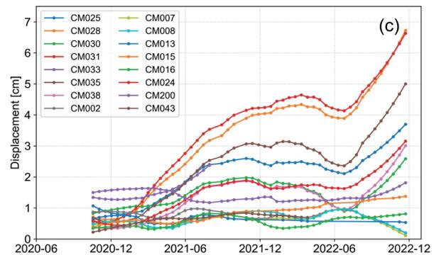
Fig. 3 - Cumulated displacement results. (a) inclinometer displacement on sliding surfaces; (b) GNSS displacements; (c) RTS displacements
