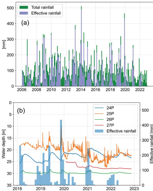
Fig. 4 - (a) Rainfall dataset and effective rainfall from Diga del Brasimone weather station (top); (b) piezometer monitoring data
