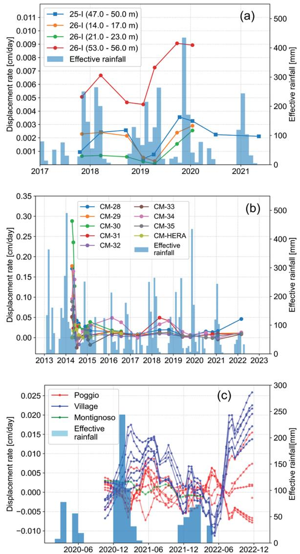
Fig. 5 - Comparison between effective rainfall time series and slope displacements provided by GNSS monitoring (a), inclinometer monitoring (b) and RTS monitoring (c).
