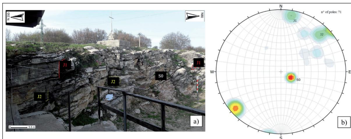
Fig. 4 - a) Field-based geomechanical scanline and identification of bedding plane (S0) and joint sets (J1, J2); b) Stereographic projection derived from the scanline survey (equal area projection, lower hemisphere)
