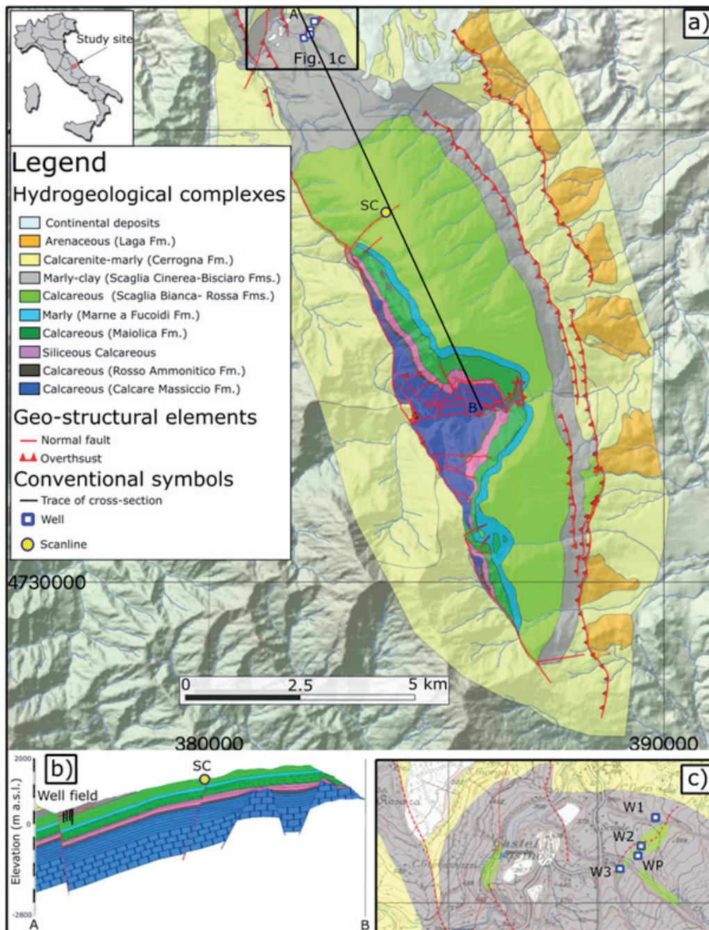
Fig. 1 - Location of the study site with a) hydrogeological map of the Montagna dei Fiori hydrostructure, with indication of wells (blue squares) and the geomechanical scanline (yellow circle, SC); b) hydrogeological cross-section (trace reported in Fig. 1a), and c) magnification of Fig. 1a for the well field area modified from TAZIOLI *et alii*, 2020
