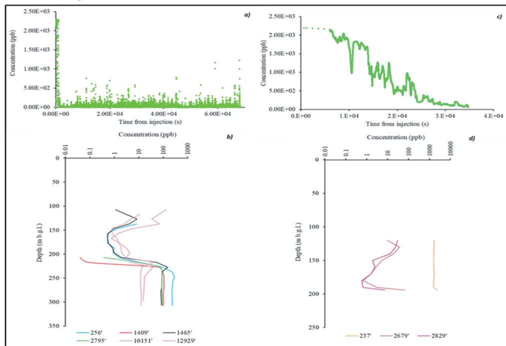
Fig. 2 - a) BTC for the TEST1; b) vertical logs for TEST2; c) BTC for the TEST3 and d) vertical logs during TEST3
