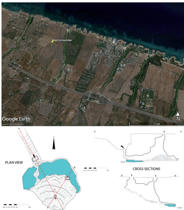
Fig. 4 - Above: Grotta Puntore location with respect to the coastline; green dotted lines represent the main traces of the ephemeral karst valleys locally named “lame”. Below: map view and cross sections of Grotta Puntore (mod. after survey by Gruppo Escursionistico Speleologico Ostunese – GEOS, on June 06, 2020); the light blue color highlights the brackish lake within the cave
