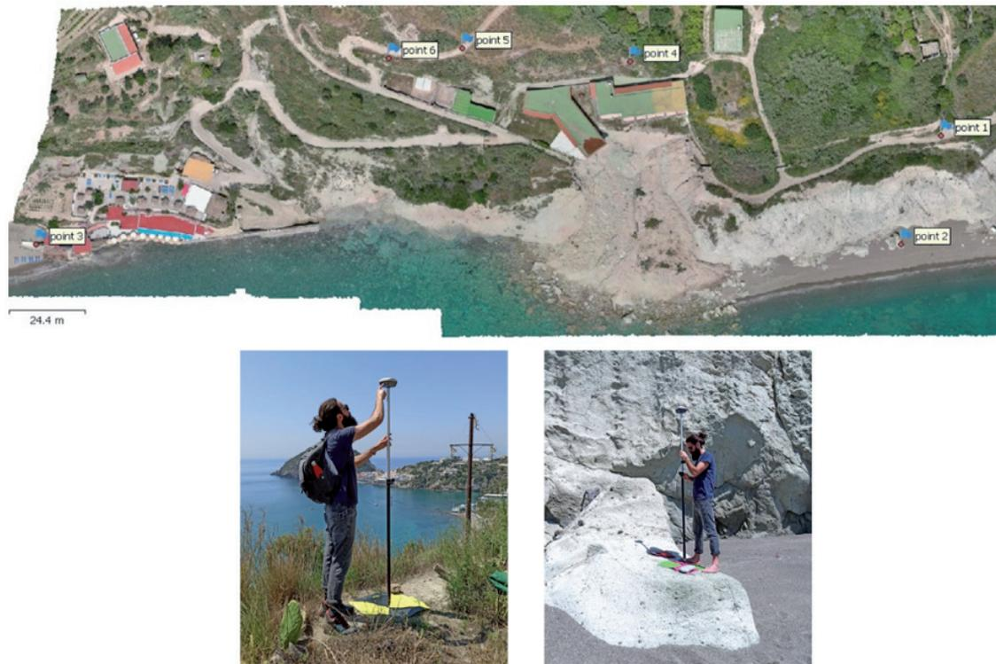
Fig. 4 - Photogrammetric targets locations (above) and example of targets measurement (point 2 – bottom right; point 6 – bottom left)
