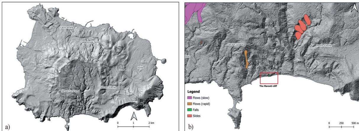
Fig. 1 - (a) The Ischia Island and (b) a zoomed view of the Maronti bay (study site in the red rectangle). Landslides affecting the area are depicted also as reported on the IFFI Project (Italian Landslide Inventory) from TRIGILA *et alii* (2010)
