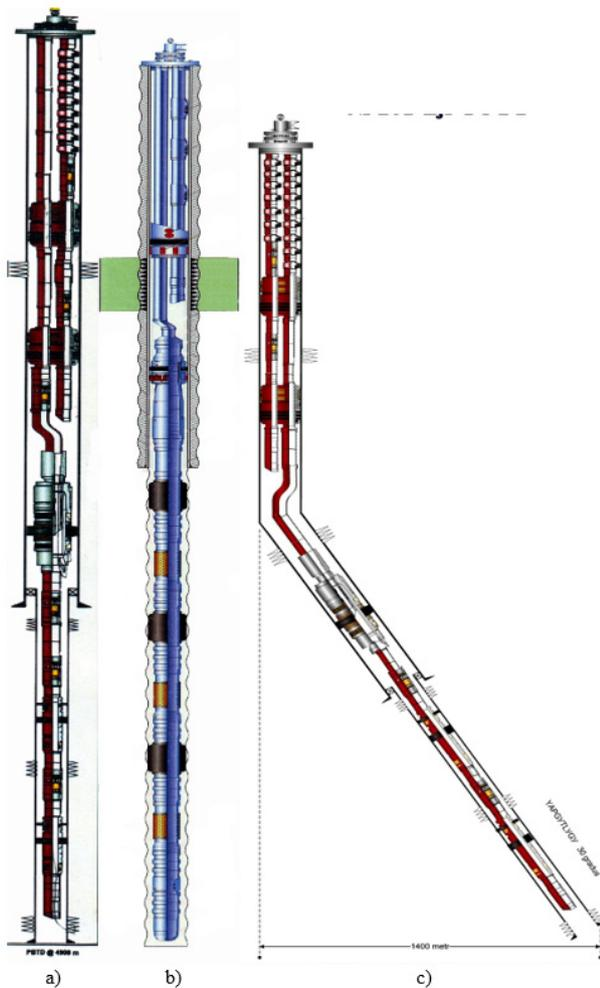
Fig. 4 - Schematic diagrams of double-lift tubing hangers: a) Well No. 37; b) Well No. 147; c) Well No. 201 (design)
