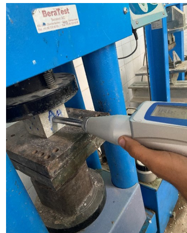
Fig. 5 - Schmidt Hammer Rebound test on the prepared limestone samples
