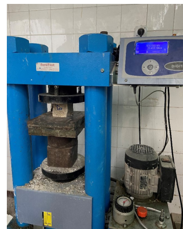
Fig. 6 - Uniaxial Compressive Strength test on the prepared limestone samples
