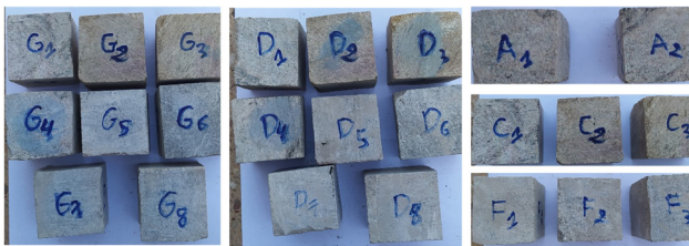
Fig. 3 - Cutting and numbering the cubes of the limestone samples
