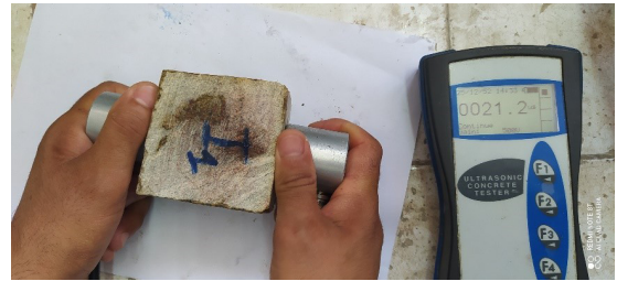
Fig. 4 - Ultrasonic Pulse Velocity test on the prepared limestone samples
