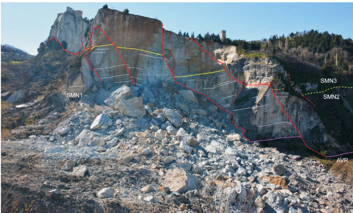
Fig. 9 - The NNE rock wall after the 2014 rockfall. The unconformable SMN2/SMN3 boundary has taken on unambiguous morphological evidence as a roof. Above this boundary, the main scarp of the 2014 rockfall was determined by a large pre-existing fracture; below the same boundary, the main scarp developed by breaching fresh rock. Laterally, the falling rock masses were released by pre-existing high-angle normal faults
