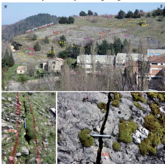
Fig. 6 - a) Trace of the main fractures on the top of the cliff (families K1, K2, K3 and K4); b) and c) details of the K3.2 fracture which belongs to the same family as the fracture of the 2014 landslide
