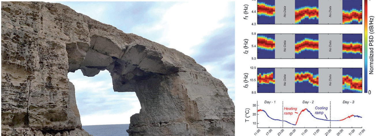
Fig. 12 - View of the Wied Il-Mielah sea arch where are visible the joints separating blocks from the arch beam. The graph on the right shows a detectable variation of the main eigenmode frequencies during a daily temperature change (from GRECHI & MARTINO, 2020)
