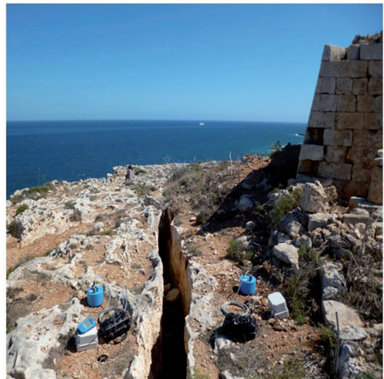
Fig. 4 - Passive seismic measurements performed at the Selmun promontory through LE-3D/5a Lennartz three-component seismometers (0.2 Hz eigenfrequency) together with REFTEK 130-01 dataloggers. The sensors were distributed astride the open joints to detect effects related to a “volume-controlled” vibrational model
