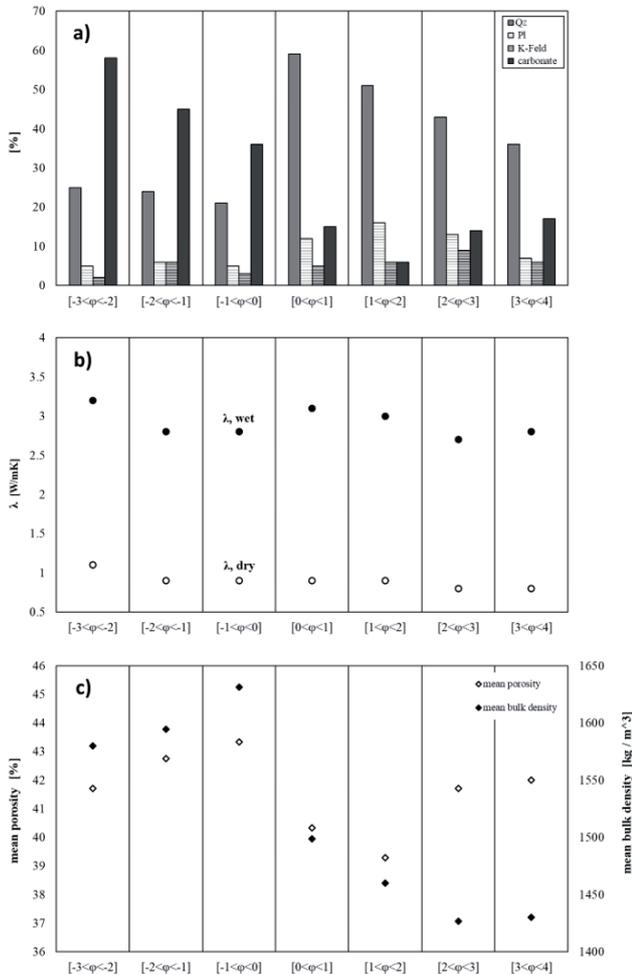
Fig. 2 - Particle size fraction versus a) mineralogical composition (%); b) average thermal conductivity in dry and wet conditions (W/m·K); and c) average porosity (%) and bulk density (kg/m<sup>3</sup>)
