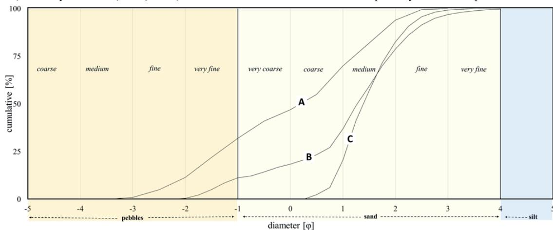
Fig. 1 - Cumulative grain size curves of no-sieved soil samples
