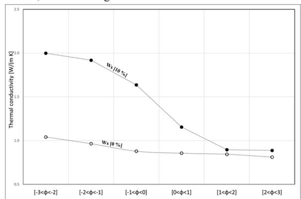
Fig. 4 - Thermal conductivity versus particle size classes for degree of saturation in water ( $W_s$ ) of 10% m<sup>3</sup>/m<sup>3</sup>
