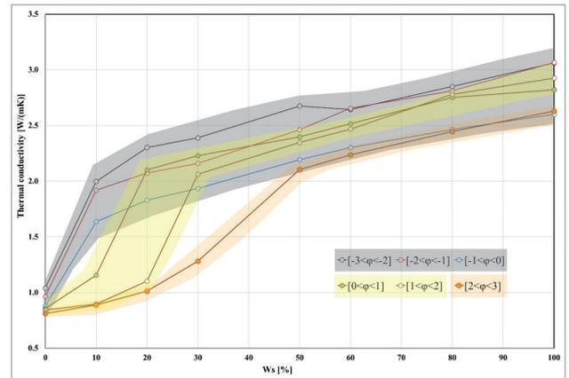
Fig. 3 - Thermal conductivity versus degree of water saturation ( $W_s$ ) in % m<sup>3</sup>/m<sup>3</sup>; for each particle size classes
