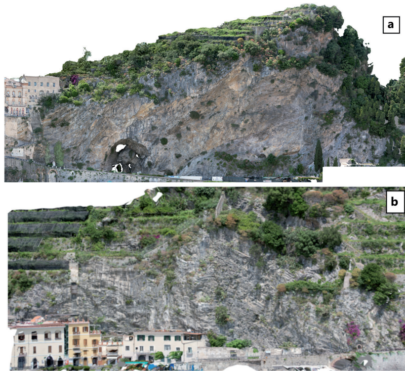
Fig. 7 - Orthomosaics depicting the slopes surveyed in localities Maiori (a) and Minori (b), and analysed by Photomonitoring techniques
