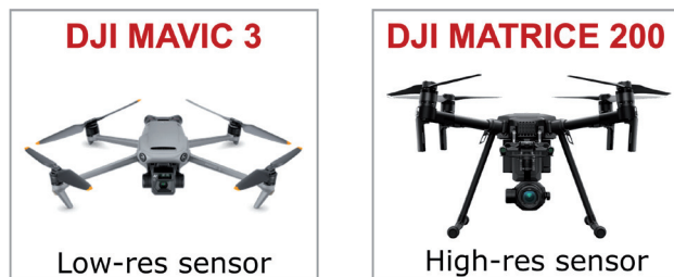
Fig. 4 - Unmanned aerial systems used for photogrammetric surveys of the rock cliffs in Minori and Maiori
