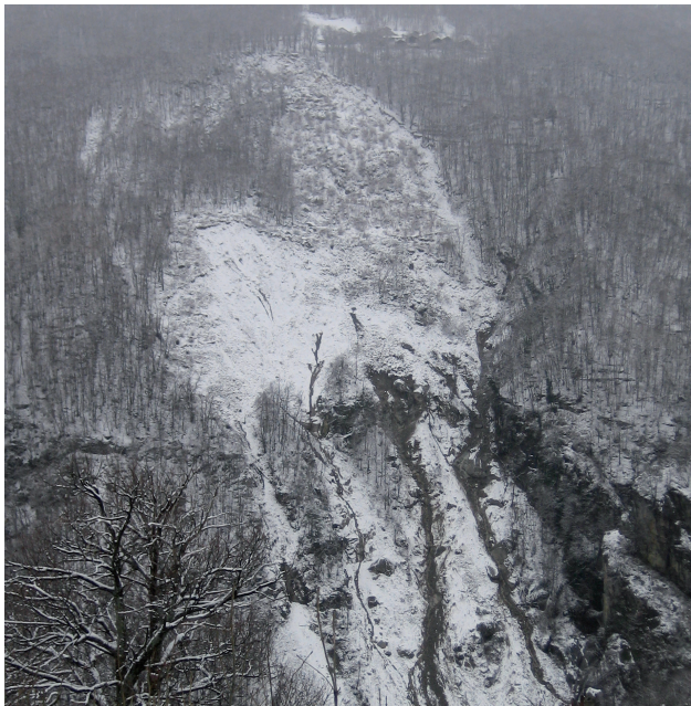
Fig. 25 - Frontal view of landslide; snow highlights springs in the lower sector
