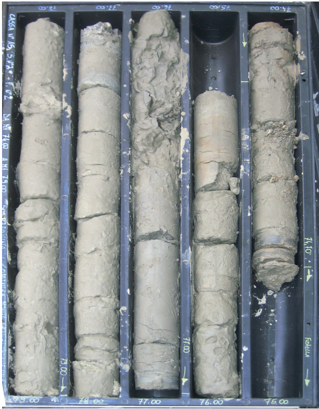
Fig. 8 - Silty layer found in the center landslide drilling at depth between 67.00 and 82.50 m
