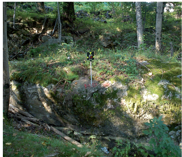
Fig. 4 - Topographic target in landslide
