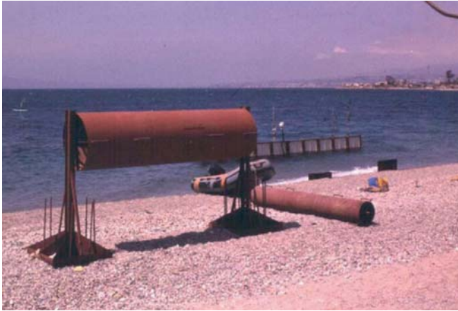
Fig. 9 - Esperimento RC1993: il modello del tunnel sommerso per l'attraversamento stabile Calabria-Sicilia - Experiment RC 1993: the model of the submerged tunnel for the jointing Calabria-Sicily
