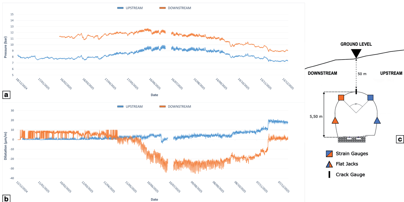
Fig. 7 - Monitoring of the stress state of the tunnel carried out through (a) flat jacks; (b) strain gauges; (c) schematic cross-section of the tunnel showing sensor locations
