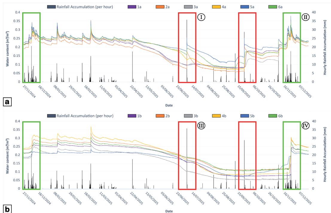
Fig. 5 - Water content measured by capacitive probes in relation to hourly rainfall accumulation. Sensors placed 40 cm above ground level (a); sensors placed 80 cm above ground level (b). The red box indicates high-intensity but short-duration rainfall events, while the green box indicates moderate-intensity but longer-duration rainfall events
