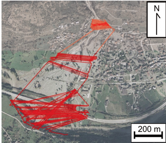
Fig. 8 - Mapping of invaded areas using the proposed volumetric method. The red lines show the envelope of the flooded areas. Background: aerial photograph of the past event.
