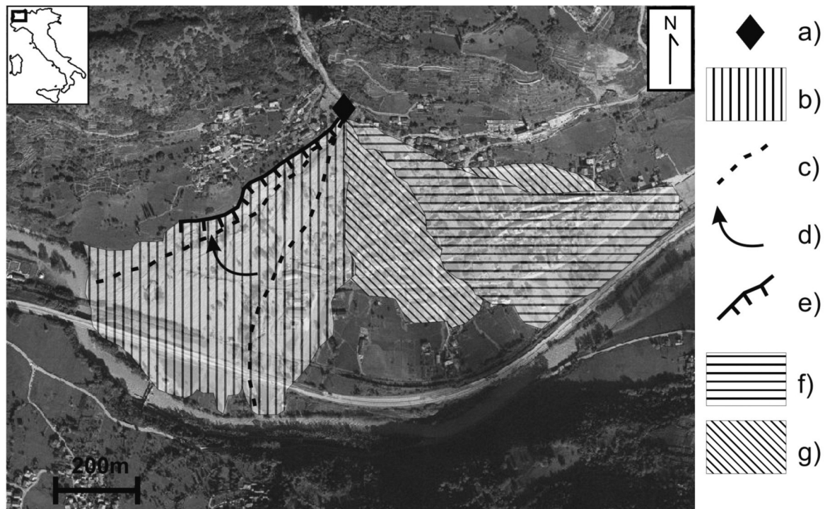
Fig. 3 - Schematic map showing the main effects of the debris-flow surveyed after the event. Key to legend: a) Location of the main obstruction point where the flow diverted into two main branches; b) Heavily flooded area with deposition of coarse grained debris (boulders and gravel), locally incised by transportation channels; c) Boundary of the sector dissected by channels; d) Migration direction of the main channel; e) erosional scarp; f) Heavily flooded area with deposition of sandy debris; g) Lightly flooded area with deposition of sandy and silty debris.
