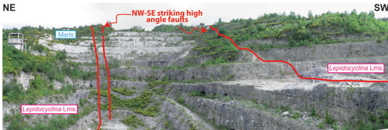
Fig. 22 - View of the Valle Romana Quarry. In the Quarry only two lithostratigraphic units of Bolognano Fm outcrop: the Lepidocyclus Limestone and the overlying hemipelagic marls. The north-eastern (left) and south-western (right) sides are affected by a two main fault zones NW-SE striking and NE dipping, that drop down the eastern block (left) with an oblique-slip kinematics.
