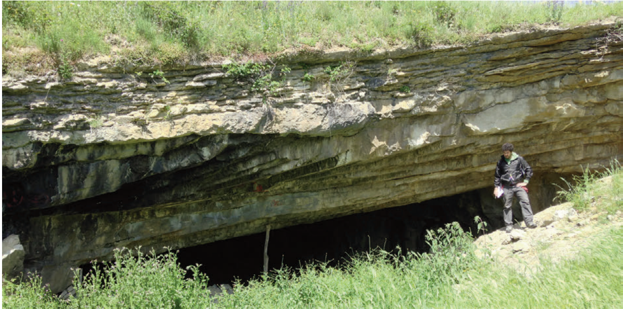
Fig. 19 - Mines excavated along strata in the upper portion of the Lepidocyclina Limestone with bitumen in matrix porosity.
