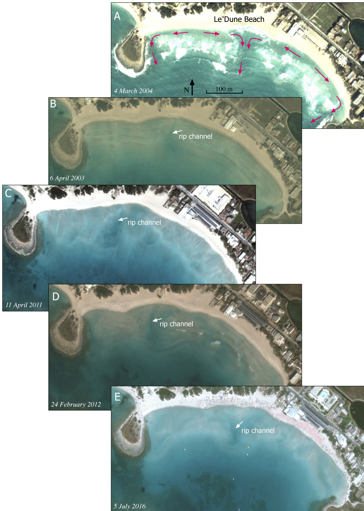
Fig. 21 - Satellite images of different periods at Le Dune beach (images from Google Earth). Possible rip circulation during a storm event is shown in A. In B-E, changes in time and space of the nearshore bar pattern with persistence of the main rip channel in the middle of the beach.
