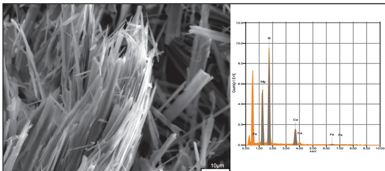
Fig. 5 - SEM/EDS analysis of asbestos tremolite (sample T2).
