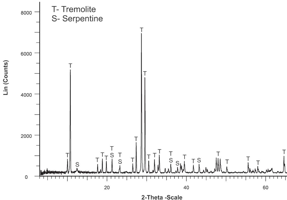
Fig. 3 - XRPD pattern of asbestos tremolite (sample T2).
