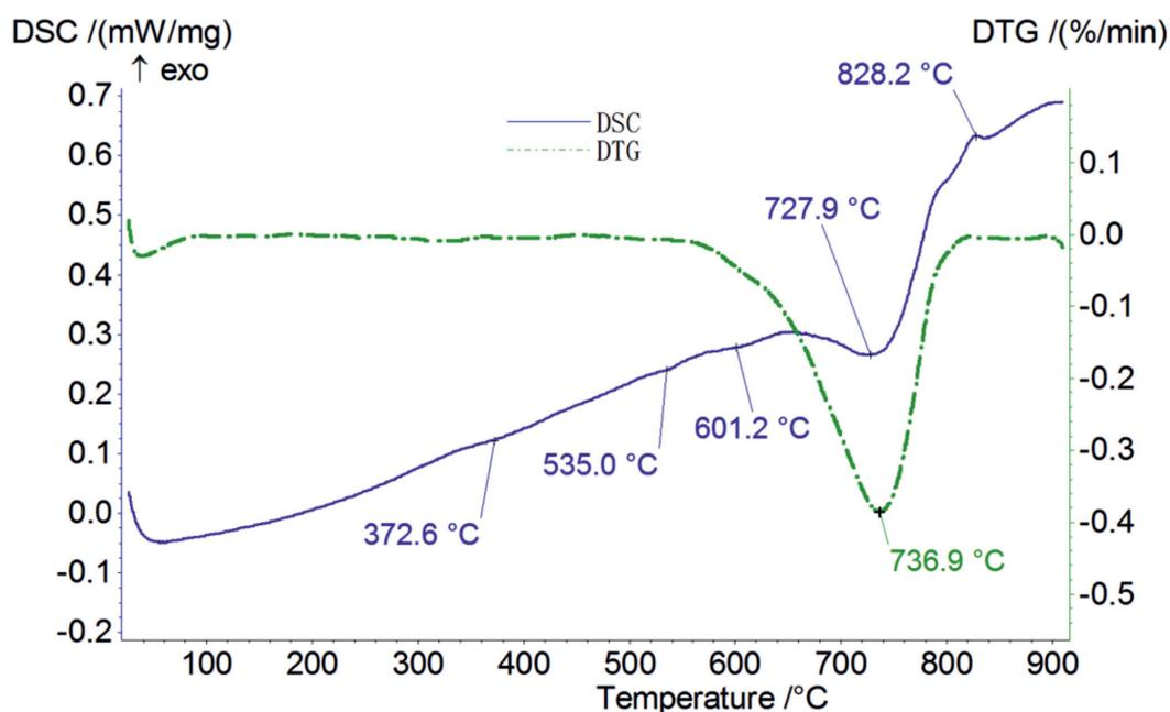
Fig. 4 - Thermal analysis of asbestos tremolite (sample T2).
