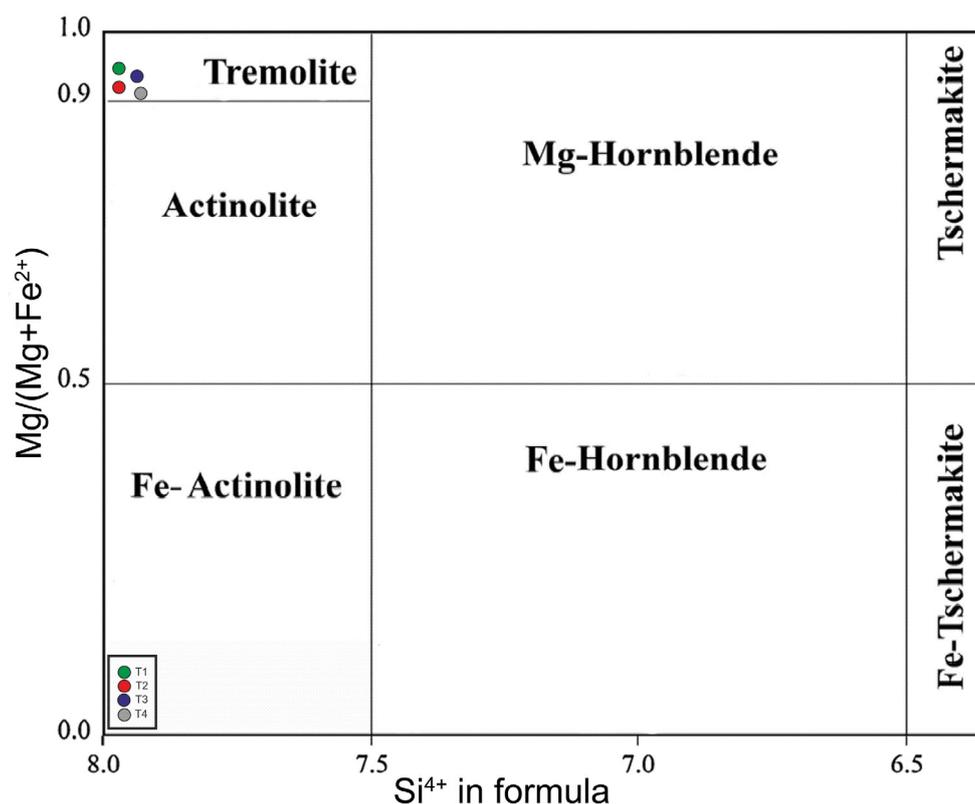
Fig. 6 - Amphibole diagram classification (after Leake et al., 1997).
