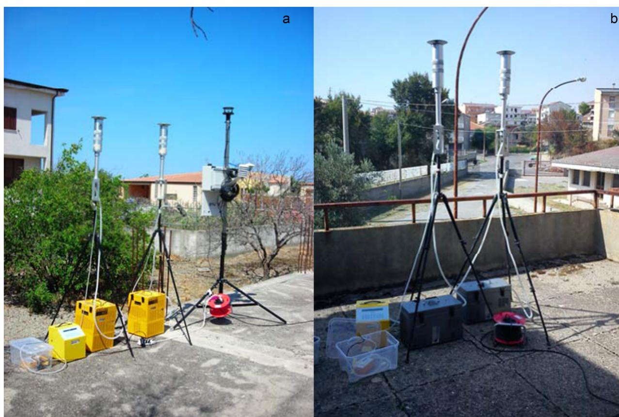
Fig. 5 - Low-flow sampling system used for the campaign Strongoli 1 at CP1 (a) and SP3 (b) stations.
