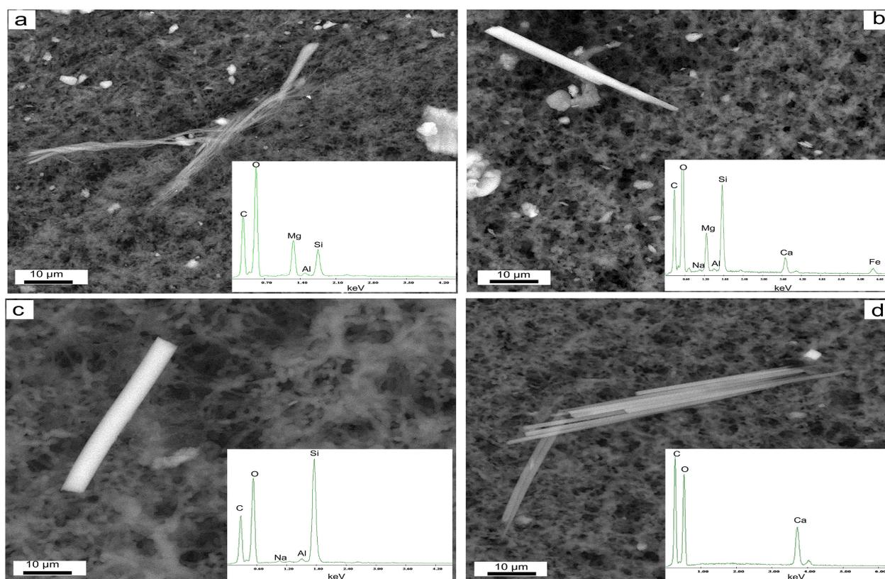
Fig. 6 - Mineral fibres of chrysotile (a), tremolite (b), silicatic glass (c), and calcite (d) with the relative energy-dispersive spectrometry (EDS) point analysis.
