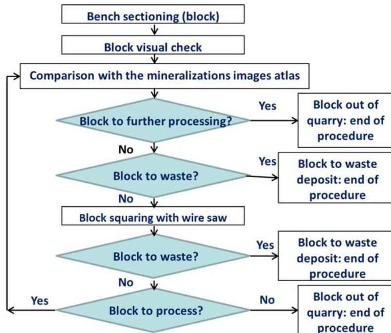
Fig. 6 - Block suitability check flow chart.
