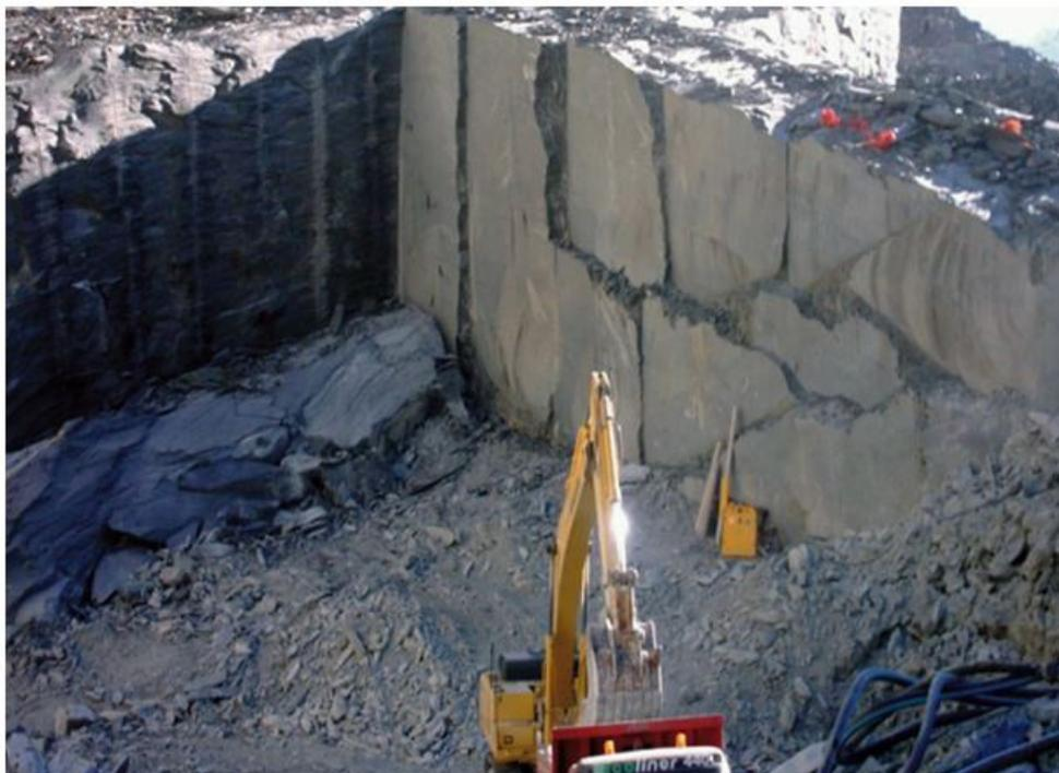
Fig. 5 - Bench splitting in Central Alps green Stones mines.
