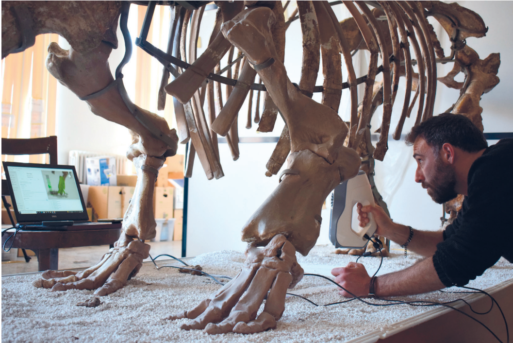
Fig. 9 - An example of digital acquisitions ongoing at MUST, laser scanning performed on a mounted skeleton of Hippopotamus with Artec Eva Scanner.
