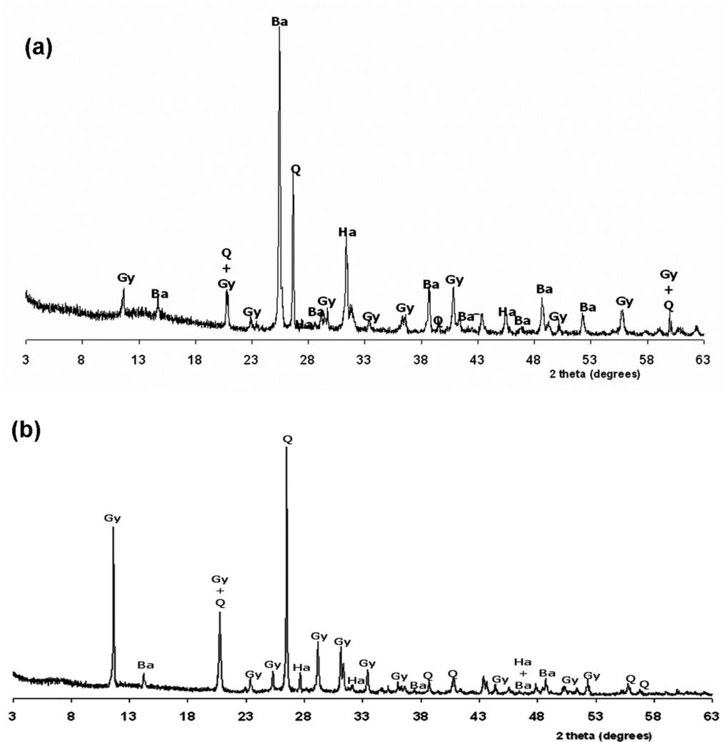
Figure 7. Representative XRPD patterns of the studied salt samples. (a): XRPD pattern of the salt layers. (b): XRPD pattern of the hard crust sample. The identified minerals were labelled as follows: Ba = Bassanite; Gy = Gypsum; Ha = Halite; Q = Quartz.
