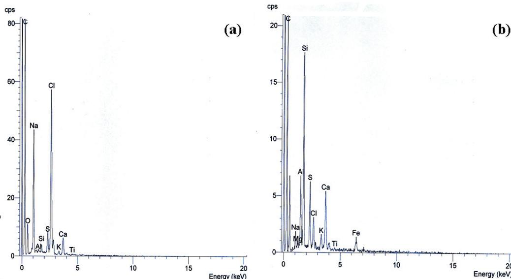
Figure 6. EDS spectra recorded on the damaged layers. (a): EDS spectrum obtained on the salt layer. (b): EDS spectrum obtained on the hard crust.
