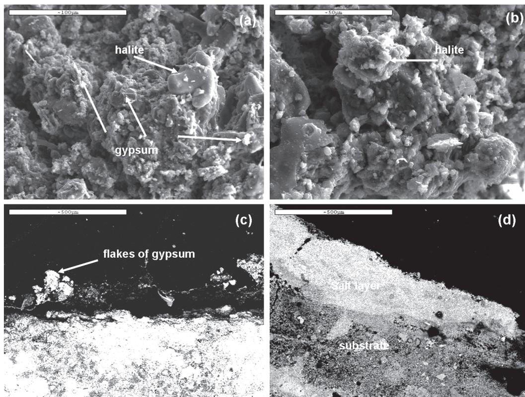
Figure 5. Some SEM and BSE micrographs obtained on the damaged layers. (a): SEM micrograph of the external surface of the hard crusts. (b): SEM micrograph of a salt layer shows the crystallization of different salts, waxy, and hollow-faced halite covers the stone surface. (c): BSE image obtained on a cross-section of the hard crusts. (d): BSE image obtained on a cross-section of the salt layer.
