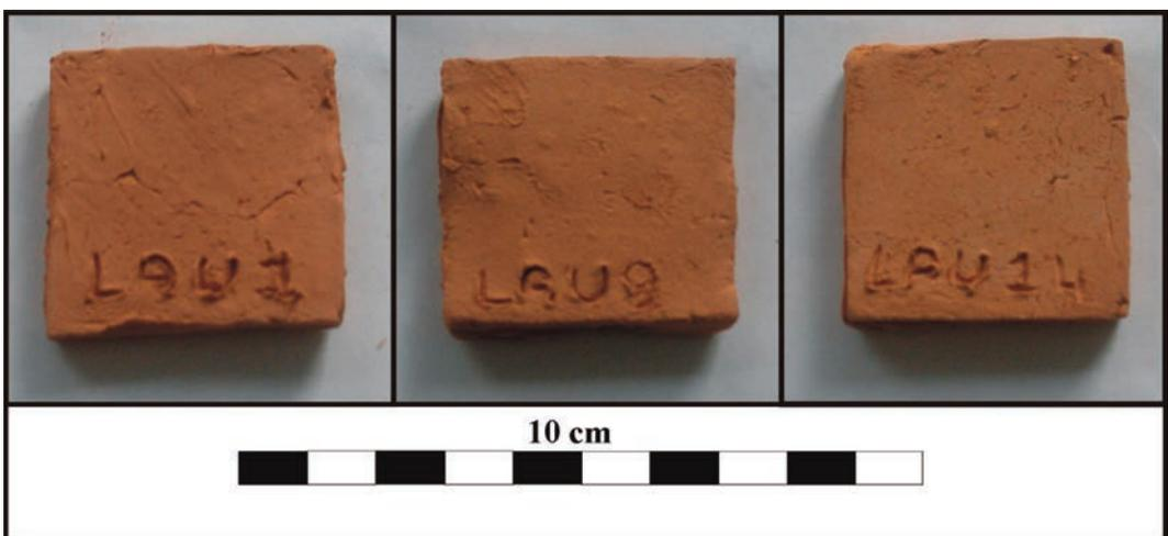
Figure 5. Experimental tests with the local clay samples fired at 950 °C.
