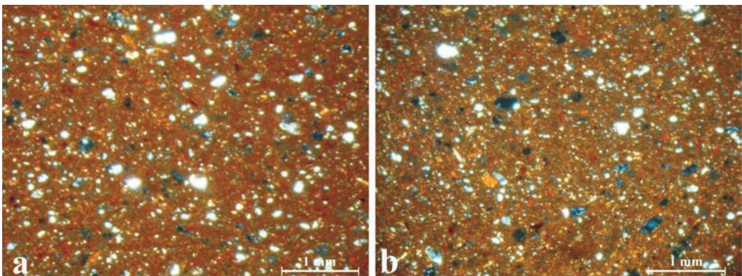
Figure 8. Thin-section microphotographs showing: a) representative matt-painted Fringe style sample (SM13); b) representative firing test of local clayey materials (LAU1). All images were taken in XPL.
