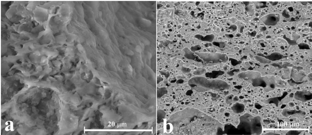
Figure 7. SEM photomicrographs of sample SM14 with initial vitrification degree (a), and over-fired sample 4/5 (b) exhibiting a continuous vitrification with bloating pores.
