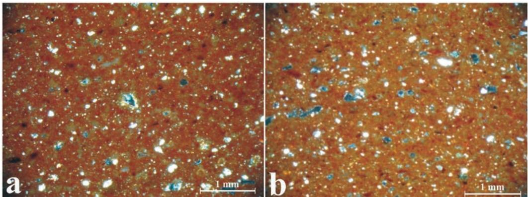
Figure 4. Microphotographs of thin sections for optical microscopy (OM) analyses under crossed nicols, showing the fabric of representative matt-painted samples: a) Undulating Band Style (sample 1/87); b) Fringe style (sample SM13). Magnification 15X.
