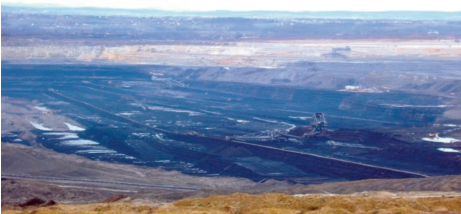
Figure 3. View of the Tamnava opencast mine and coal exploitation. Removal of the overburden generates large amounts of dust, whereas in the case of actual coal mining (middle bottom) no visible dust is generated.
