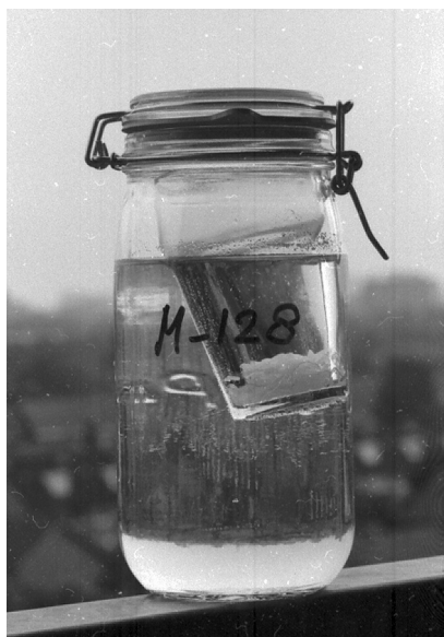
Figure 2. Hermetically sealed jam-jar filled with CO_2 -saturated water to which magnesium (metal) powder had been added; the floating beer glass contains KOH pellets needed to absorb the dissolved carbon dioxide.
