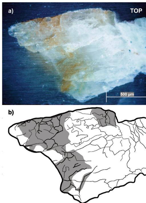
Figure 5. a) Cross section from the top of sample PC 2 down to 1mm inside the granitic substrate; b) line drawing highlighting the location of the iron-rich compounds (in grey).
