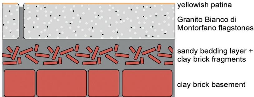
Figure 2. Stratigraphy of the Piazza Cavalli. From bottom to top (not in scale): 15<sup>th</sup> century brick basement in a sandy mortar; 10 cm-thick sandy mortar bed with earthenware pieces inside; Granito Bianco Montorfano flagstones; a few-micron thick yellowish patina.
