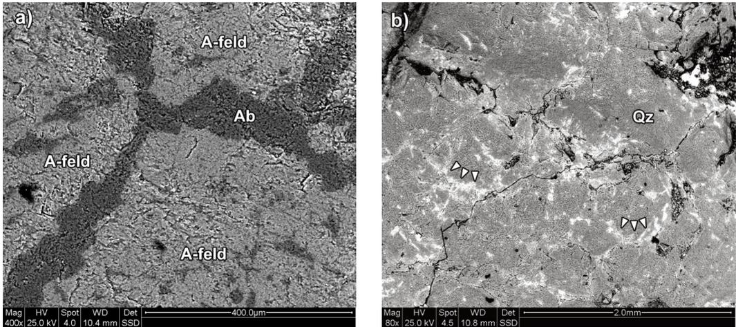
Figure 6. a) BSE image showing the micropores on feldspars. A-feld = micropertthite; Ab = albite; b) BSE image showing the enrichment of iron along grain-grain contacts (arrows). Qz = quartz.
