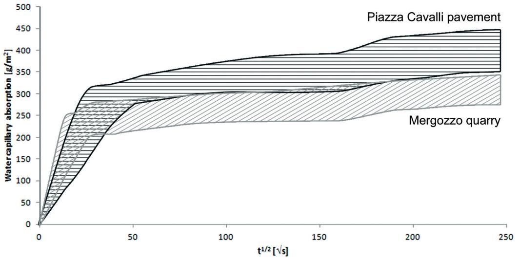
Figure 8. Comparison of capillary water absorption curves between five granite cores from Piazza Cavalli (hatched area) and eight granite samples (crosshatched area) quarried in 2010 at Mergozzo (NW Italy).
