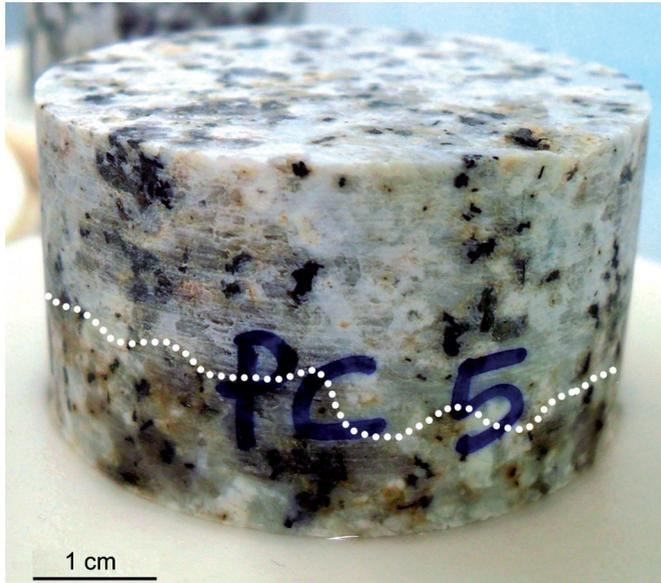
Figure 7. Capillary wetting front visible during the water absorption test for the core PC5.
