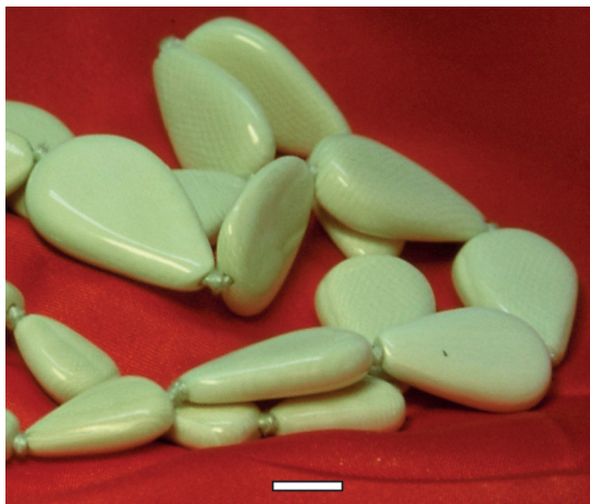
Figure 1. Characteristic “engine-turning” surface pattern of elephantine ivory (from a necklace, the scale bar corresponds to 1 cm), showing criss-crossing continuous Schreger lines (“X” type) and obtuse intersection angles.
