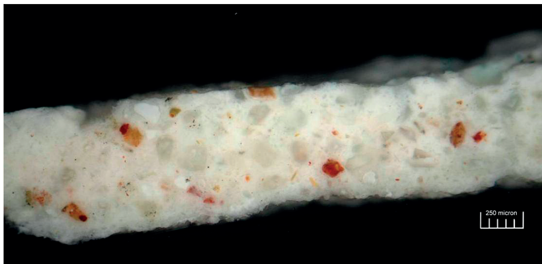
Figure 3. Cross section image of the adhesion mortar.
