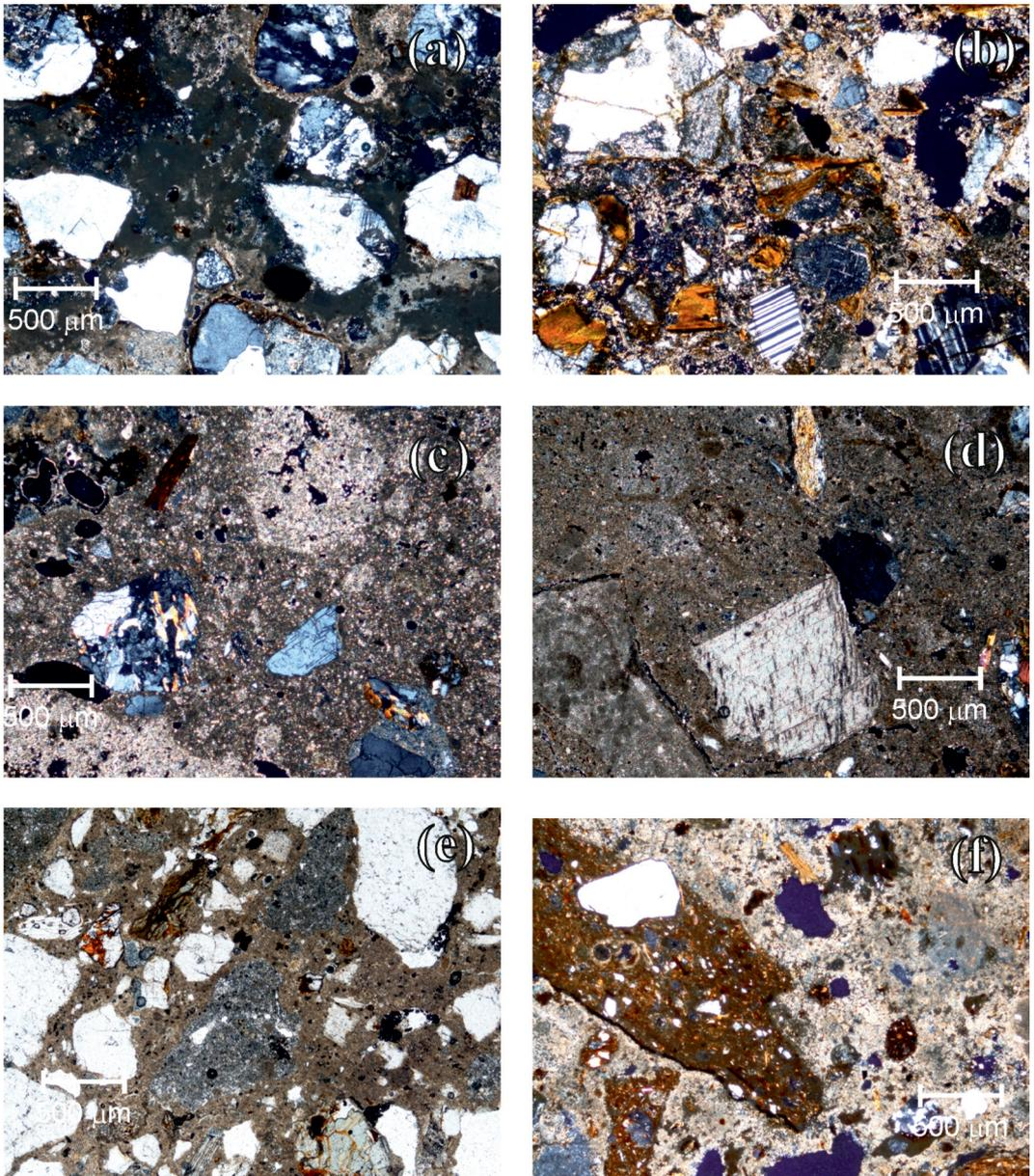
Figure 4. Microphotographs of plasters and mortars: (a) high degree of thickening and micritic binder in sample TA19; (b) very heterogeneous aggregate in sample TA21; (c) lumps in sample TA6; (d) spar calcite in the binder in sample TA7; (e) aggregate in sample TA8; (f) grog in sample TA11.
