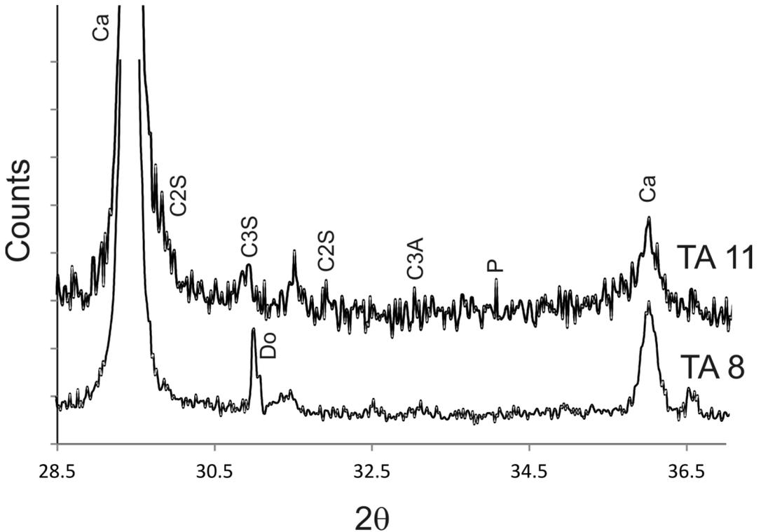
Figure 6. X-ray diffractograms of samples TA8 and TA11: Ca = calcite; Do = dolomite; C2S = belite; C3S = alite; C3A = tricalcium aluminate; P = portlandite.
