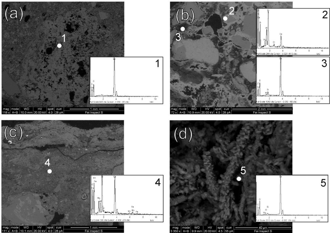
Figure 5. SEM images of plaster and mortar samples: (a) lump and Ca-rich binder in sample TA6; (b) millimetric chemical variation in binder in jointing mortar sample; (c) high content of  $\text{SiO}_2$ ,  $\text{Al}_2\text{O}_3$ ,  $\text{Fe}_2\text{O}_3$  in samples with grog; (d) hyphae of lichens associated to calcium oxalate and halite in sample TA7.
