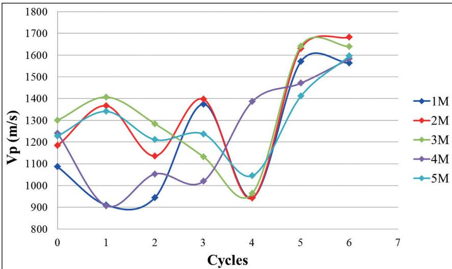
Figure 11. Velocity of the ultrasonic P-waves measured on the samples during crystallization test.
