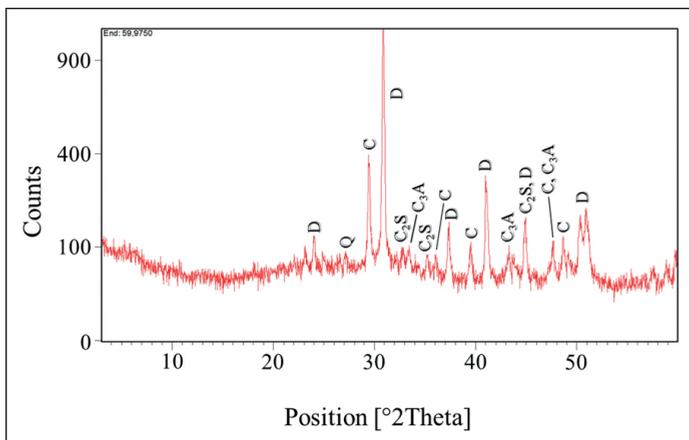
Figure 7. XRPD spectrum of the mortar (whole sample). D = dolomite; C = calcite; C<sub>2</sub>S = dicalcium silicate; C<sub>3</sub>A = tricalcium aluminate; Q = quartz.
