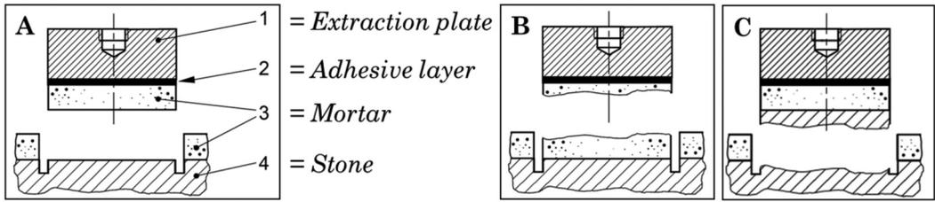
Figure 8. Different types of fractures that can occur by the adhesive strength test. A) fracture at the interface between the mortar and the support; B) fracture within the mortar; C) fracture within the support.
